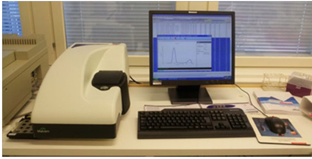
Figure 1: Photography representation of Malvern zeta sizer used for finding particle size & zeta analysis
