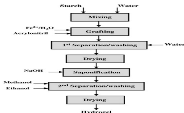
Figure 7: Block Diagram for the Preparation of the High Swelling Hydrogel
